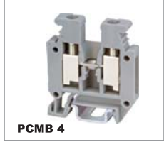
PCMB 4 CE 500V/32A 0.2-4mm 2 UL 300V/30A 10-26AWG T/W/End plate 6.2/28/1.5mm
