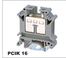
PCIK 16 CE 400V/76A 4-16mm 2 UL 300V/85A 12-4AWG T/W/End plate 12.2/42.5/1.8mm
