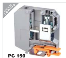
PC 150 IEC 1000V /309A 50-150mm 2 UL 600V/285A 2-300MCM T/W/End plate 31/100/-mm
