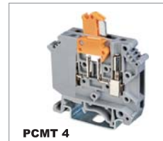
PCMT 4 CE 800V/16A 0.2-4mm 2 UL 600V/16A 24-12AWG T/W/End plate 6.2/51/-mm
