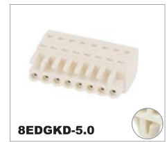
8EDGKD-5.0 CE 320V/20A 0.2-2.5mm 2 UL 300V/15A 22-14AWG Poles 2P-24P
