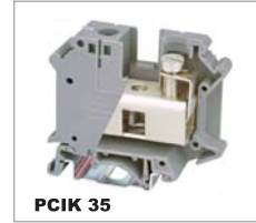
PCIK 35 IEC 600V/125A 0.75-35mm 2 UL 600V/115A 18-2AWG T/W/End plate 15.2/55/-mm
