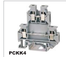
PCKK4 CE 500V/32A 0.2-4mm 2 UL 300V/30A 26-10AWG T/W/End plate 6.2/56/2.6mm
