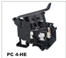
PC 4-HE CE 800V/6.3A 0.2-4mm 2 UL 600V/12A 24-12AWG T/W/End plate 8.2/72.5/-mm
